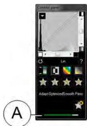
Ideal image quality is achieved when the Control Panel exposure indicator is a full green bar. This example shows the RVG 6200 Control Panel with exposure indicator (A). Avoid under-exposed or over-exposed images indicated by a partial or full red bar:
