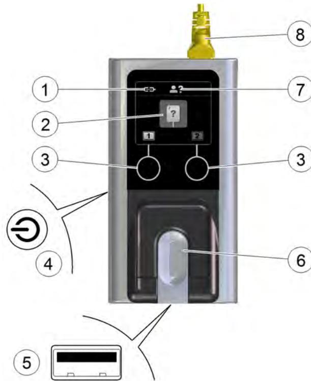
1 Indicates whether the RVG Connect unit is paired with the workstation:
